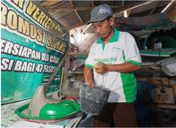
▲ A trained sanitation entrepreneur is producing toilet pans
