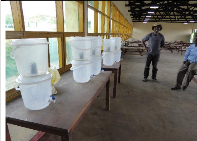
The ADPP school who used water filters. After a good start the filters are now not being used. A reason is lack of organization of maintenance
