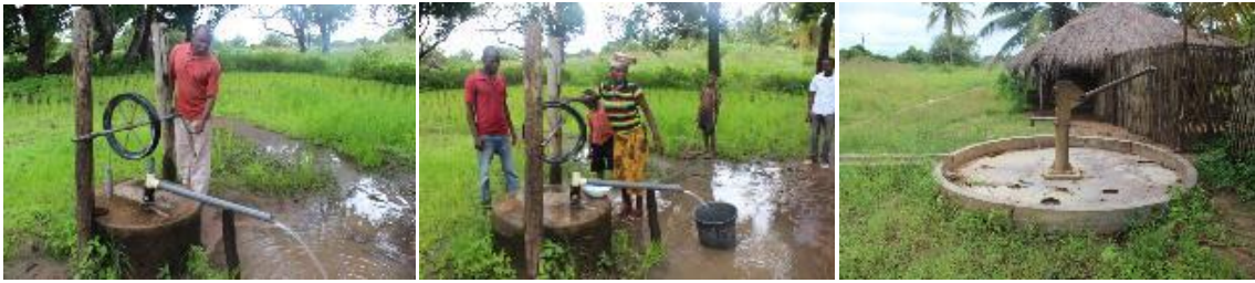
Picture 10: A water hole opened by FACT/ADPP in 2007 ( on the left ) and a broken Afridev water pump ( right ). This water hole is not only being used for the horticulture field irrigation, but even to get water for drinking.
